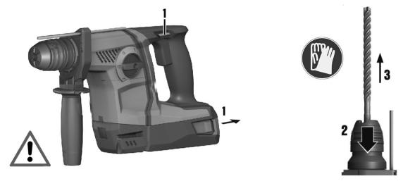
Pull the chuck back as far as it will go and remove the accessory tool.
