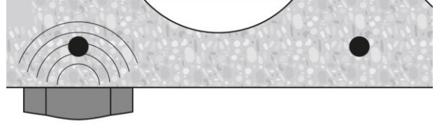
2. Positioning pre-stressed steel
